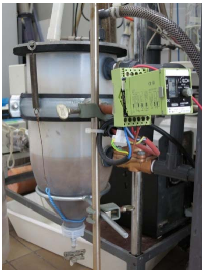
Figure 2-3: Secondary clarifier with timer.
