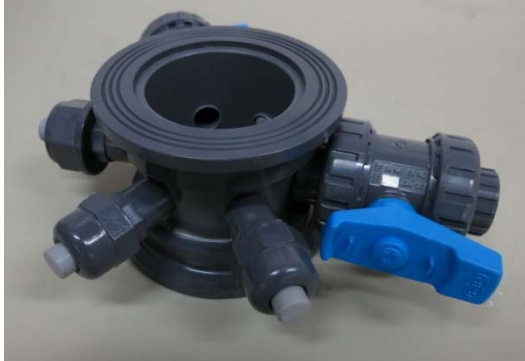
Figure 2-2: PVC section with apertures for the installation of probes.
