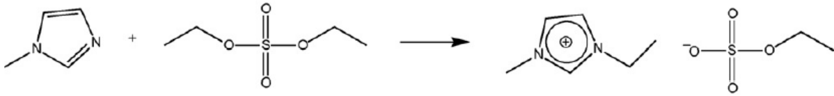
Figure 3.5: Synthesis of the Ionic liquid 1-ethyl-3-methylimidazolium ethylsulfate.
