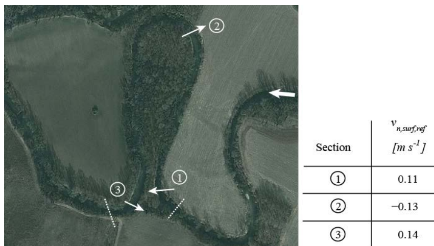
Figure 5 Bend on the Ledra River (Italy, Image: Google Earth) and maximal v_{n,surf,ref} computed with Blanckaert and de Vriend's model (2003; 2010). The dashed lines indicate the domain of the numerical simulation. The white arrows indicate the location of the maximum values of v_{n,surf,ref} .
