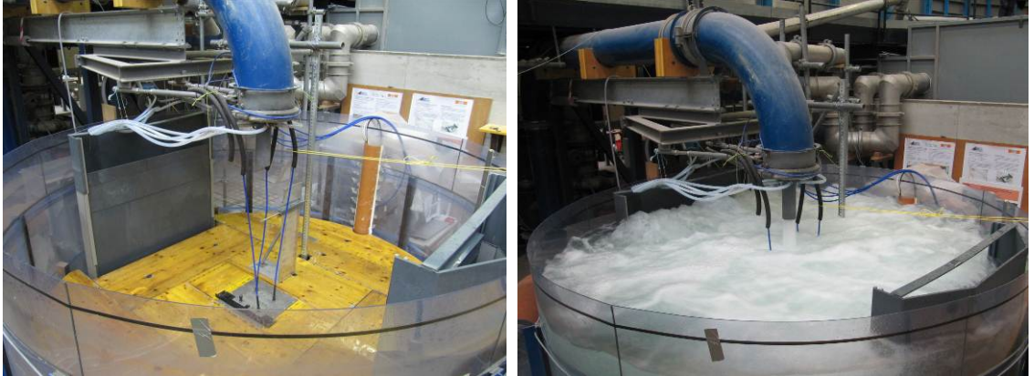
Figure 2 Pictures of the experimental facility before and during tests. In the left picture the fixed confined block can be seen in the middle
