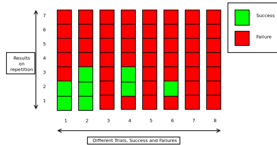
Fig. 3. Unreliability of the system. We repeated the same input 7 times on our set up in consecutive trials and observed their results. This was done for 8 different starting points– successes and failures. We observed that there is never a success after four consecutive iterations. Success could be obtained by starting from success as well as failed initializations. These results are due to the highly noisy and unreliable nature of our set up.
