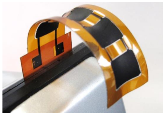
Figure 35 – DEMES made with single membrane and Kapton tape adhesive layer
