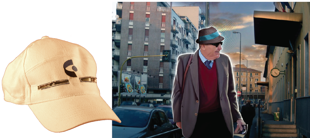
Figure 1.1: VisionHat , a wearable electronic travel aid system designed to extend mobility of blind and visually impaired people by providing collision-alert feedback (left); concept application - VisionHat supports visually impaired person in outdoor navigation.
