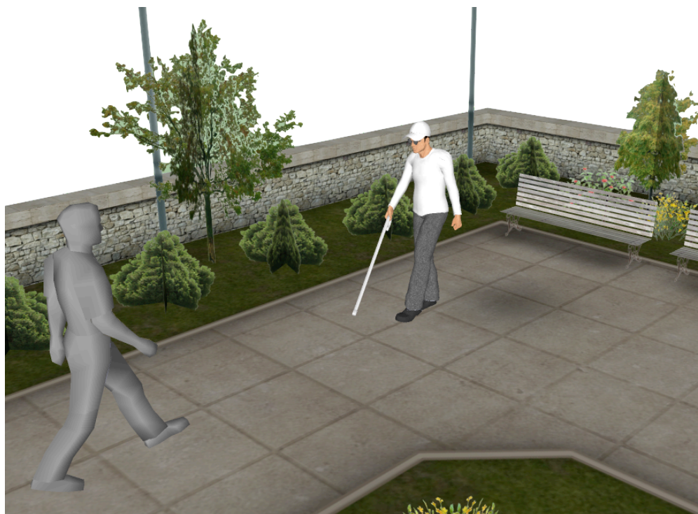
Figure 5.14: Experiment 2: outdoor walking during a cloudy day. The aim of the experiment is to show the performance of the VisionHat system during outdoor operation. The user, typically equipped with a white cane as well as the VisionHat , is walking with an average speed of approximately 1 m/s. An approaching person is passing by with a speed of approximately 1.5 m/s at a distance of approximately 0.5 m. The experiment is conducted under cloudy-day light conditions with an average illuminance of 850 lux, as measured on the ground level.
