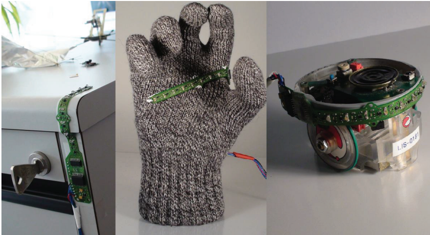
Figure 2.3: Examples of Vision Tape integration onto various substrates. Wooden cupboard (left), wool glove (middle), polymeric turret of wheeled robot [47] (right).
