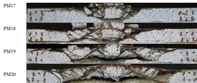
Fig. 10—Saw-cuts after post-punching regime of specimens with bent-up bars.
