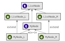
**Figure 4.** An example of miniboxed class inheritance. The suffixes are: M - miniboxed encoding and L - reference type. Compare to the specialized class inheritance in Figure 3.
