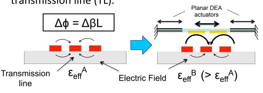
Moving the conductor strips laterally over the TL, using planar dielectric elastomer actuators (DEAs), varies the change in  $\epsilon_{eff}$  and therefore the phase  $\phi$  by the relationship above.
