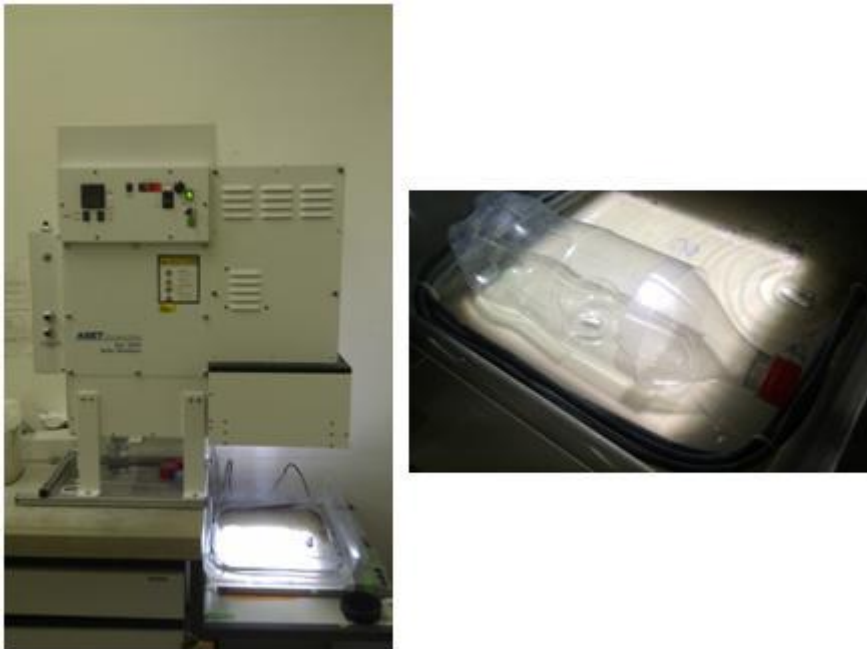
Figure 5 : experimental set-up. Solar simulator (left) and PET bottle with a beaker inside exposed to the light from the simulator (right)
