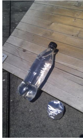
Figure 9 : Setup of the experiment done outside. Spiked water in a PET bottle and in a beaker as a dark control exposed to sunlight
