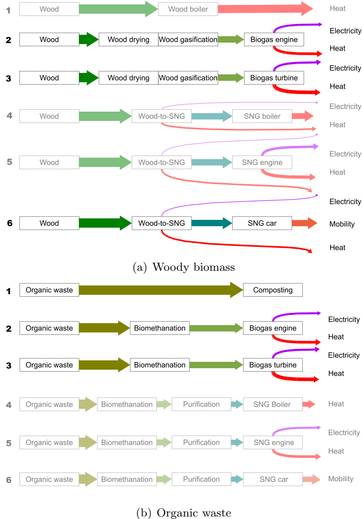
Figure 11: Selected pathways in the optimal configurations of the Pareto curve for biomass conversion: (a) woody biomass (b) organic waste. The suboptimal non-selected pathways are shaded.
