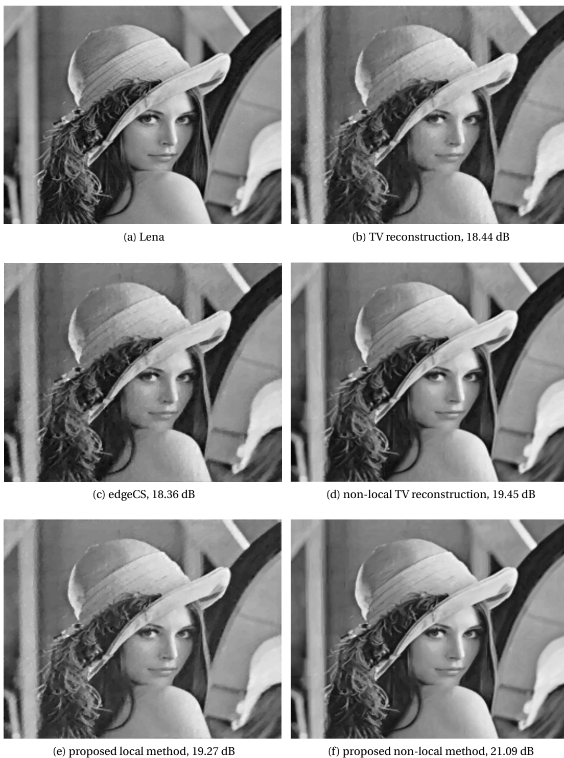
Figure 1.6: Compressed sensing reconstruction of Lena from 20% of measurements in Fourier domain.
