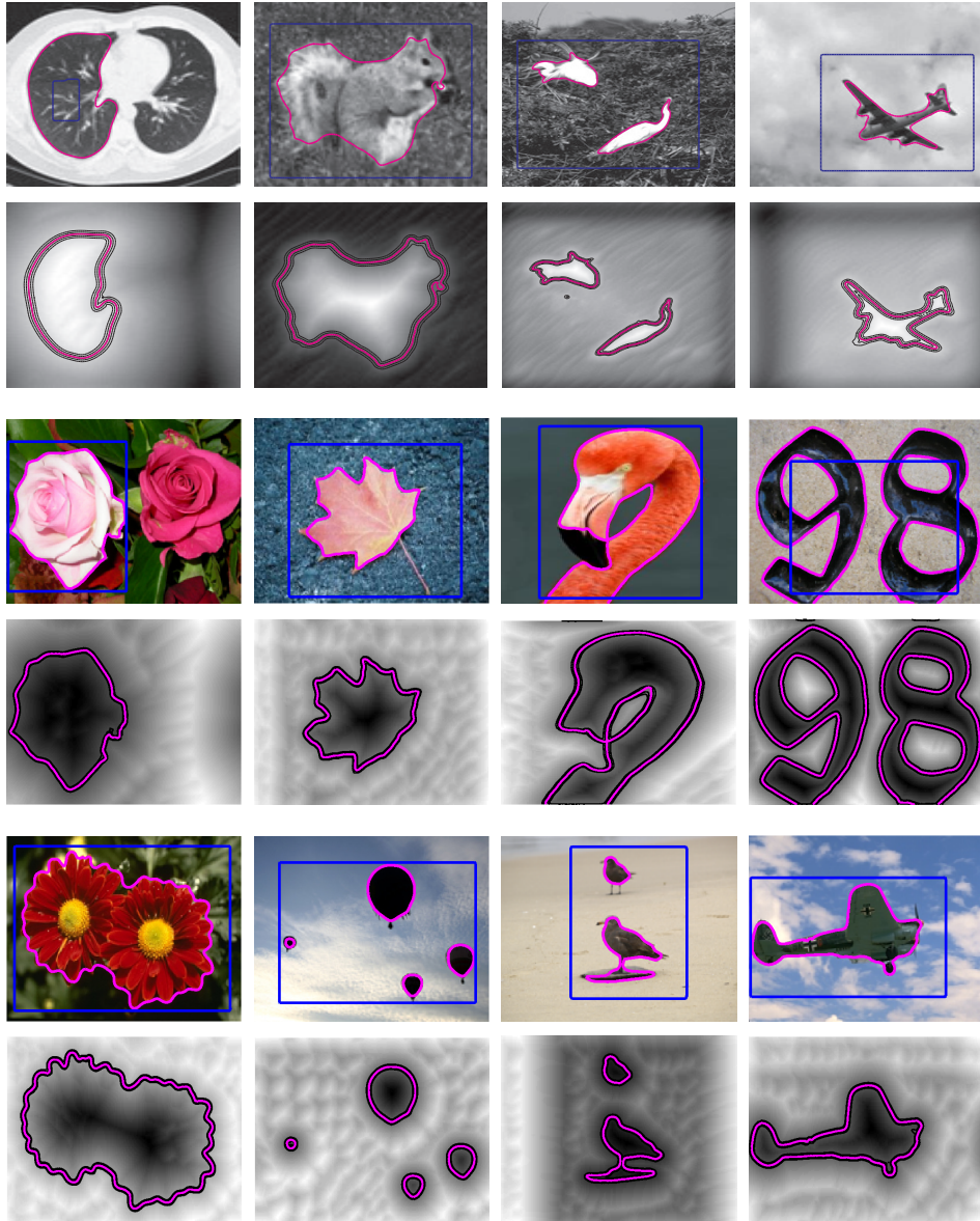
Figure 4.2: Proposed level set-based segmentation method applied to natural images. For each result, we show the segmentation result and the level set function. We plot the initial zero level set in blue, the final contour in pink and the \pm 1, \pm 2 level sets of the final function in black.
