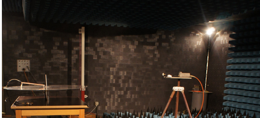
Figure 5.9 Experimental setup. Notice the SWO on the left and the D-dot connected to the fiber optic transducer on the right. On this picture the sensor is 1.2 m above the ground floor, which is 20 cm higher than the actual height of the sensor during the measurements.
