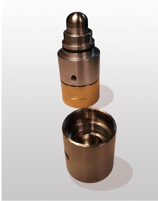
Figure 5.5 The realized prototype with the external electrode removed. Notice the inner electrode and part of the inner conductor of the main coaxial line. Notice also the sealing O-ring and the supports for the gas inlets in the wall of the coaxial line.
