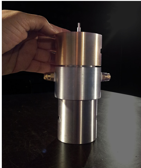
Figure 5.6 The assembled SWO. Notice the outer electrode, the outer coaxial conductor with the two gas inlets and the outer conductor of the secondary coaxial line.
