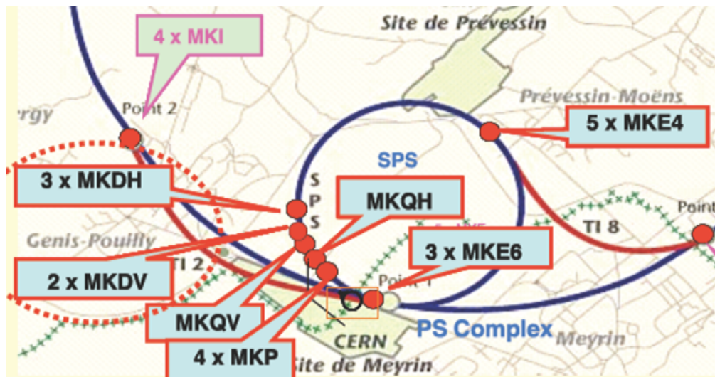
Figure 2.1: Physical locations of the SPS kickers (red dots). We can observe that the SPS kickers are not evenly distributed along the ring but are clustered around the injection zone (4 MKP), extraction zones to TI2 and TI8 (5+3 MKE), the tune measurement zone (MKDH+MKQH), and the beam dump (3 MKDV + 2MKDH). Courtesy M. Barnes.
