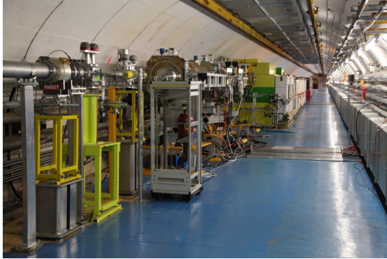
Figure 3: The TPSG experimental setup. The beam arrives from the left of the picture, the beam dump is in the background. The exact configuration of the TPSG4 and MSE was reproduced, using two separate vacuum tanks spanning over the full length of the experimental facility (9 m).
