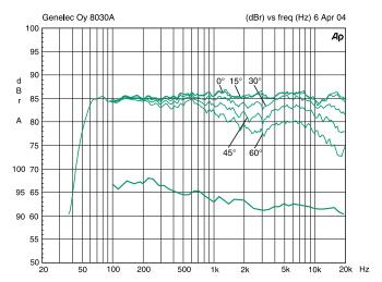
Fig. S2. The upper curve group shows the horizontal directivity characteristics of the 8030A measured at 1 m. The lower curve shows the system's power response.
