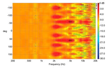
Fig. S3. Directivity sonogram of D12A polar response with 1° resolution. Measurements made at 1 m distance.
