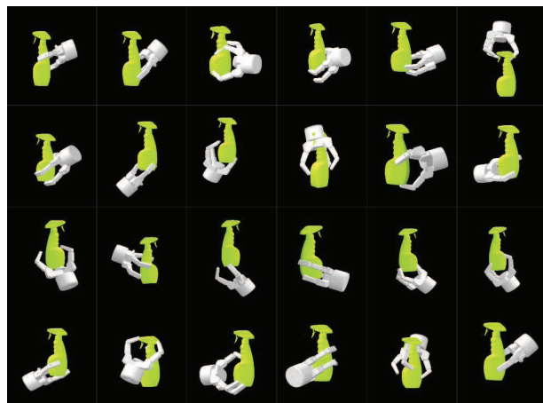
Fig. 1: typical grasps for Barrett hand grasping a spray flask
