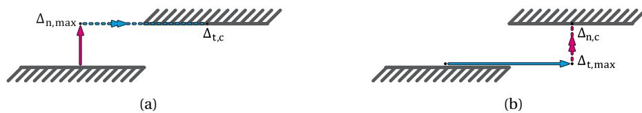
Figure 5.4: Interface non proportionally loaded: (a) first in normal direction until \Delta_{n,max} and then broken in shear and (b) first in tangential direction until \Delta_{t,max} and then broken in normal direction as in [Von den Bosch 05].
