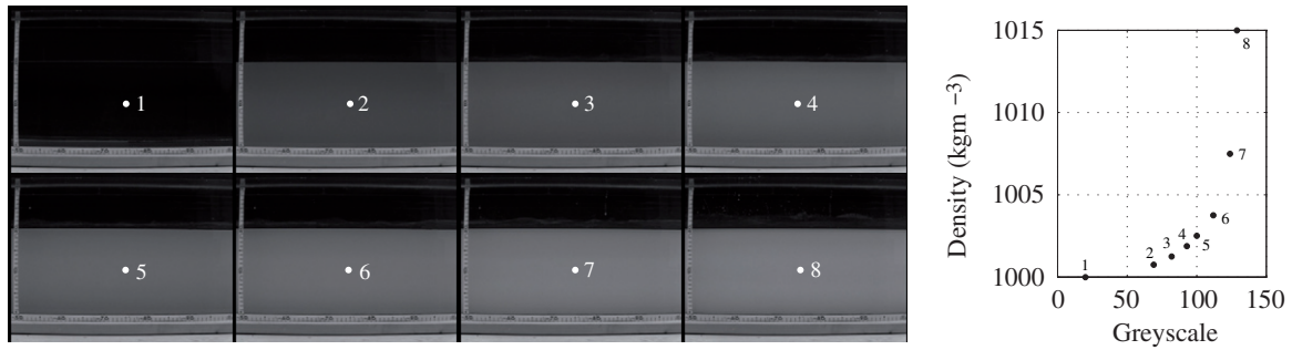
Figure 2. Example of images used for calibration and the corresponding calibration curve. The reference point corresponds to one central pixel of the image and is represented in the frames by white dots.
