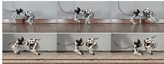
**Figure 1:** Active (top) and fixed (bottom) spine locomotion.
