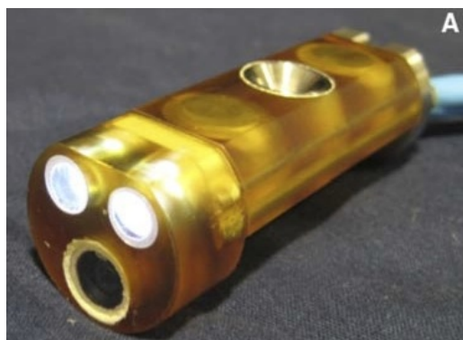
(C) MAGS camera with two LED lights
