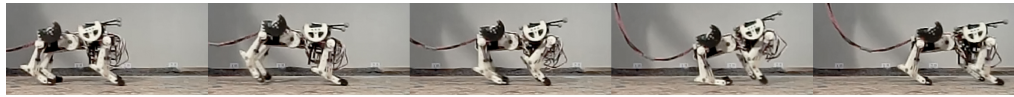
(a) Snapshot series of Bobcat-robot bounding with a fixed spine joint. This gait accelerated the robot to 0.62 \text{ m s}^{-1} . Gait cycle frequency is 3.5 \text{ Hz} .
