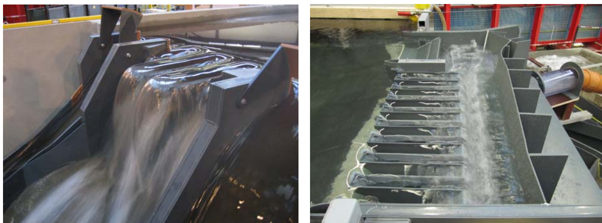
Fig. 2. Examples of physical PKW models at LCH; left: Saint-Marc Dam combining a PKW with a steep chute; right: Gage II Dam combining a PKW with a side channel. Both schemes are operated by EDF
