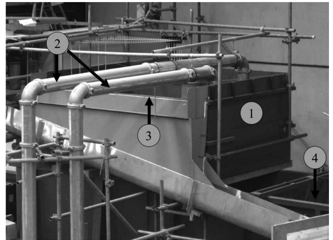
Figure 4 Setup generating positive and negative surge waves. ① Upper basin, ② water supply pipes and ③ spillway crest placed on ④ experimental flume
