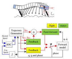
Figure 1: The schematic of the monoped model and control architecture.
