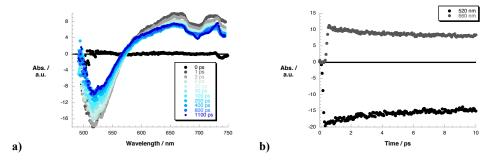
**Fig. 1.** a) Differential absorption spectrum obtained upon femtosecond flash photolysis ( $\lambda_{exc} = 480 \text{ nm}$ ) of a film of **KM-2** on 3 µm thick TiO<sub>2</sub> with the ground-state transient bleaching between 480 and 560 nm and the TA<sup>++</sup> cation beyond 580 nm. b) Time-absorption profiles illustrating the charge separation.
