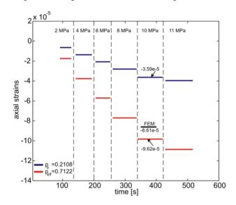
Interestingly, if only the lateral surface is loaded and the circular sections are free, the numerical simulations give B = -2.1310 and Equation (6b)  $p_e^{eff} = -0.6069$  which indicates that since the axial strain is not dominant, Equation (4a) is not appropriate. Comparing this case with that of the epoxy block, described in Section 4.1, the main difference here is the much greater elastic modulus of the glass which limits the axial strain in the core.
