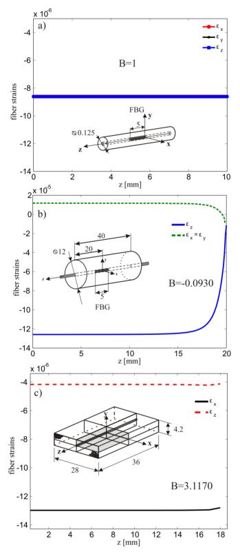
In the same Figure the corresponding prediction of the FE model at a pressure of 10 MPa is also reported. Note that use of the corrected formulation (Equation 6a) dramatically reduces the error in the determination of the fiber axial deformation. In fact, the simplification introduced considering the lateral deformations equal to  $-v_f \varepsilon_z$  generate an underestimation of the deformation by ~170%.
