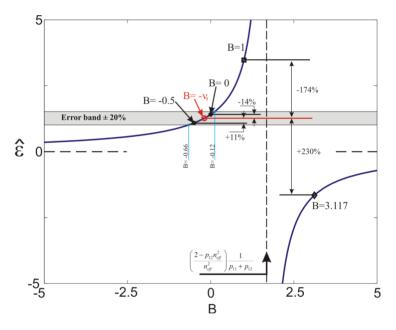
To examine the effects of relatively large lateral strains on the FBG sensor, the transversal strains are assumed homogeneous and equal ( $\varepsilon_x = \varepsilon_y$ ) but they are not related to  $\varepsilon_z$  by a simple Poisson's relation but by a *biaxiality ratio* defined as:
