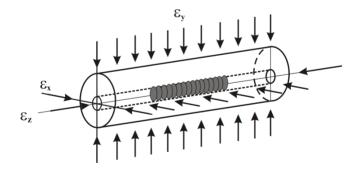
In most cases of practical interest, the FBG is subjected to axisymmetric homogeneous strains, *i.e.*,  $\varepsilon_x = \varepsilon_y$ . Assuming further that the lateral strains are related to the axial one by a standard Poisson relation  $\varepsilon_x = \varepsilon_y = -v_f \varepsilon_z$ , Equation (1) is reduced to the following simplified relation:
