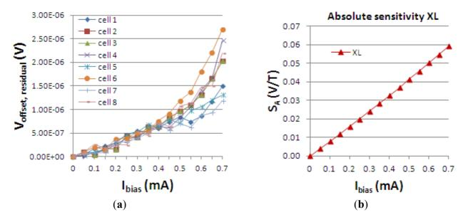
In particular, the residual offset mathematical function of the biasing current has a quadratic dependence, for the 2-phases spinning current [9]. The same quadratic increase of the residual offset with the biasing current is also observed by Demierre [10] in the Hall plate. In our case (Figure 1(a)), for 4-phases spinning current, as expected, the thermoelectric contribution proportional to  $I_{bias}^2$  in the residual offset, cannot be completely compensated for  $I_{bias} > 0.5$  mA.
