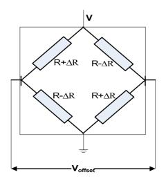
Therefore, the offset voltage caused by an asymmetry of the bridge is given by:
