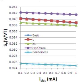
Figure 21. Voltage-related sensitivity of the simulated Hall Effect devices.
