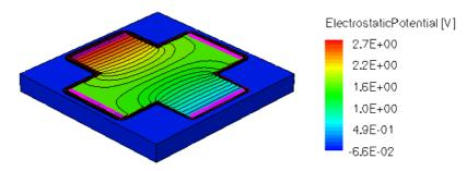
Figure 11. Electrostatic potential (V) for borderless structure, B = 0.5 T.
