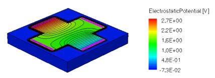
Figure 10. Electrostatic potential (V) for XL structure, B = 0.5 T.
