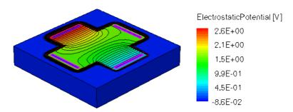
Figure 8. Electrostatic potential (V) for basic structure, B = 0.5 T.
