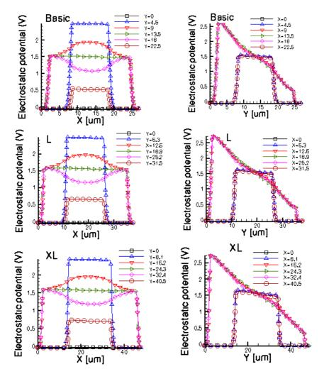
Figure 15. Electrostatic potential (V) in orthogonal cuts on Oy and Ox for optimum and borderless structures.
