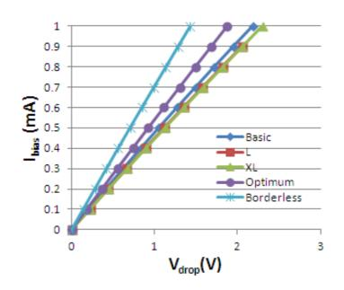
Figure 7. The simulated Hall devices I-V characteristics.
