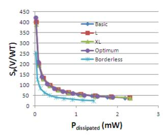
**Figure 22.** Power-related sensitivity *vs.* the dissipated power for the simulated Hall Effect devices.
