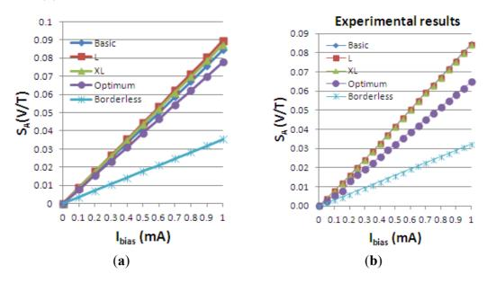
Figure 20. Current-related sensitivity of the simulated Hall Effect devices.
