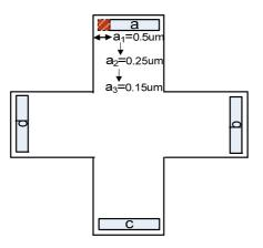
As the offset is a random process, a possible location was presumed on the contact *a*. However, other asymmetries can be induced on the rest of the contacts, as desired.
