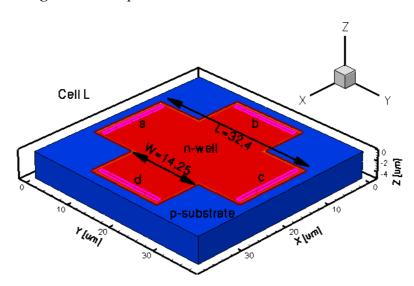
Figure 3. 3D representation of the L simulated Hall cell.
