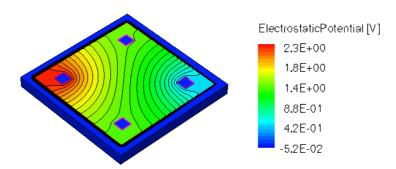
Figure 12. Electrostatic potential (V) for optimum structure, B = 0.5 T.
