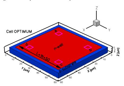
Figure 6. 3D representation of the optimum simulated Hall cell.
