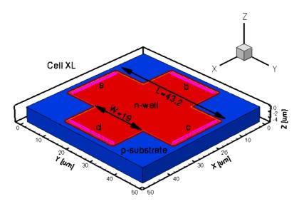
Figure 5. 3D representation of the borderless simulated Hall cell.
