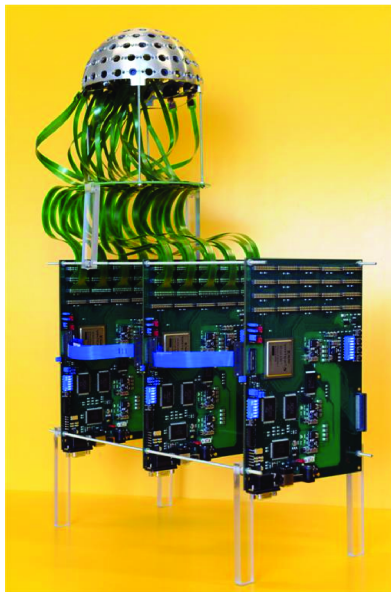
Figure 2.5: Setup of the FPGA platform for the 7-floor Panoptic system with 30 embedded cameras.
