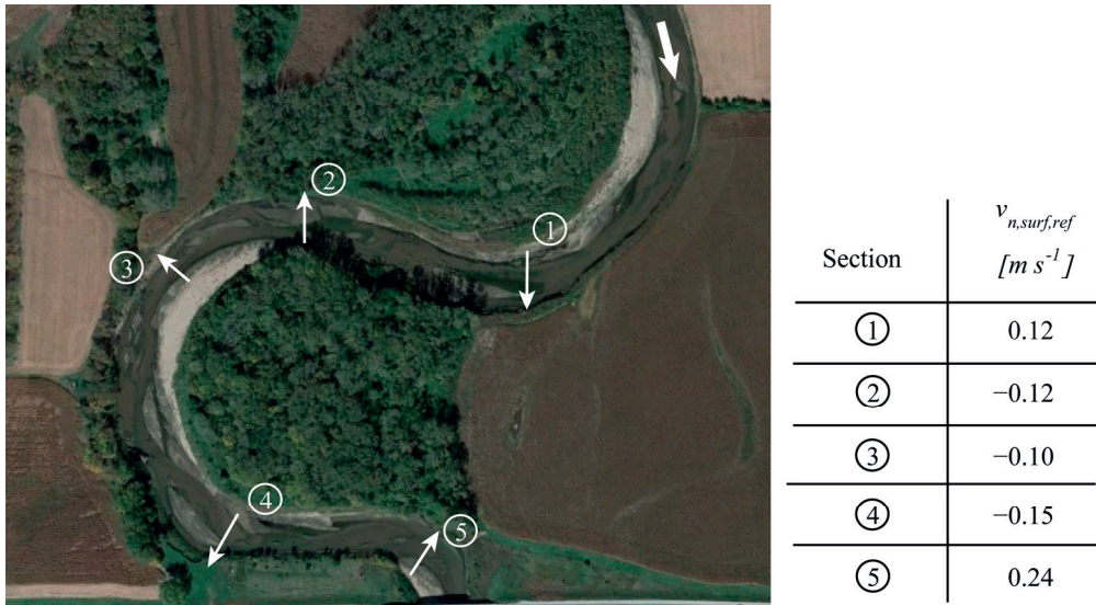
Figure 7.10: Bend on the Nishnabotna East river (USA, Image: Google Earth) and maximal v_{n,surf,ref} computed with Blanckaert and de Vriend's model (2010). The white arrows indicate the location of the maximum values of v_{n,surf,ref} .
