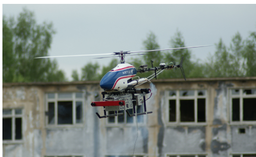
Figure 1. Unmanned helicopter ARTIS (Autonomous Helicopter Testbed for Intelligent Systems), 2 m rotor diameter, 1.5 kW 2-stroke engine, 14 kg MTOW.
