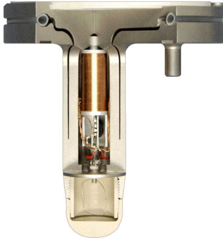
Figure 2.3: Knee instrumented prosthesis proposed by Bergmann's group. http://jwi.charite.de/en/research/ .
