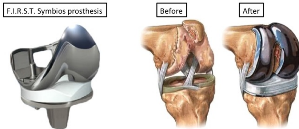
Figure 3.1: Modern artificial knee comprising the Cr-Co-Mo femoral and tibial components and an Ultra High Molecular Weight (UHMW) Polyethylene (PE) insert, and an illustration of the knee structure before and after TKA (picture modified from A.D.A.M., Inc. - http://www.healthcentral.com/rheumatoid-arthritis/9494-146.html ).
