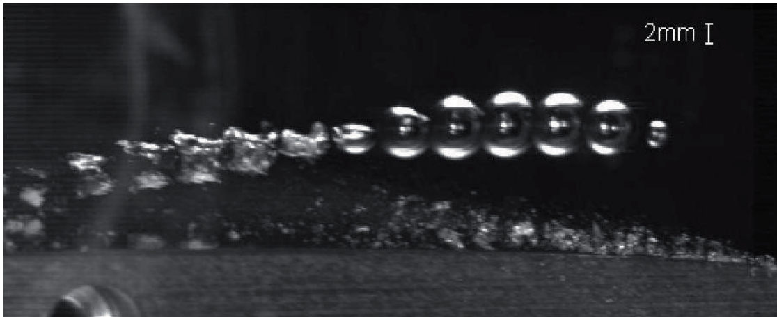
Figure 3.16: Case 2: Collapse of a bubble above the hydrofoil. The collapse is not spherical, it is initiated at the top of the bubble. Interframe time: 200 \mu\text{s} , maximum diameter: 7 mm, bubble lifetime: 1.28 ms.
