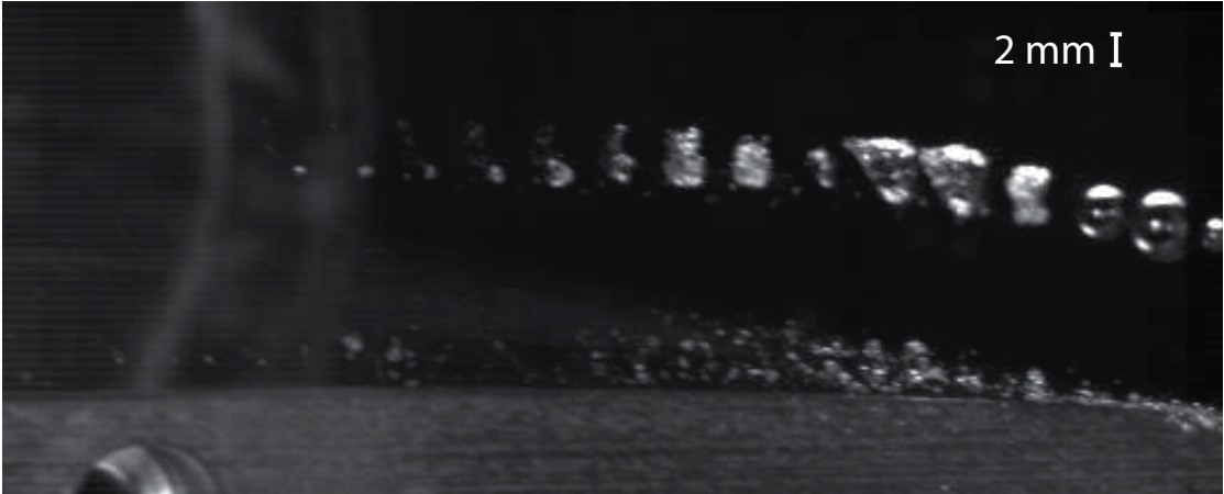
Figure 3.18: Case 3 : Superposition of the high speed images of the collapse of a bubble generated at (-5, +9). The bubble bubble has a microjet not towards the solid surface. Interframe time: 180 \mu s, maximum diameter: 5 mm, bubble lifetime: 440 \mu s.
