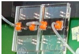
Figure 2. Differential microfluidic system showing the NIs sample (top) and the reference sample (bottom) connected in series.
