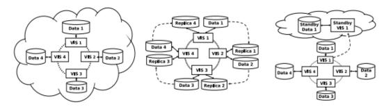
Figure 2.3: The Vis-à-Vis [114] system with 3 different storage environments: cloud, P2P storage of desktops, and a hybrid storage.
