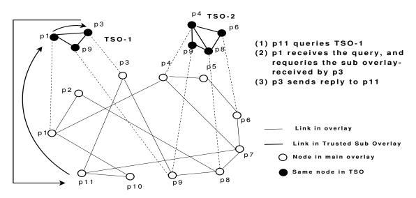
Figure 3.2: Illustration of Trusted SubOverlays.
