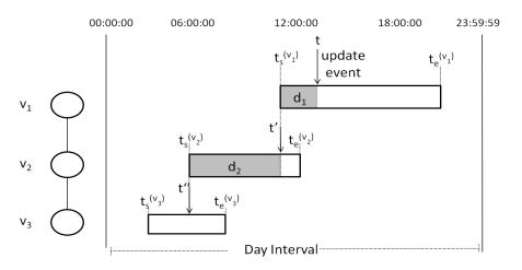
Figure 5.1: Illustration of the replica time-connectivity graph and the propagation of update from replica  $v_1$  to  $v_3$ .
