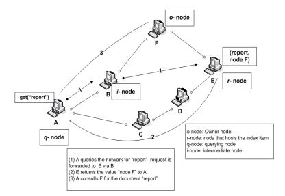
Figure 3.1: A typical message flow in a structured P2P system.
