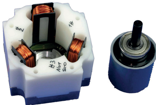
FIGURE 3.23 – Realized plastic stator and plastic rotor.
