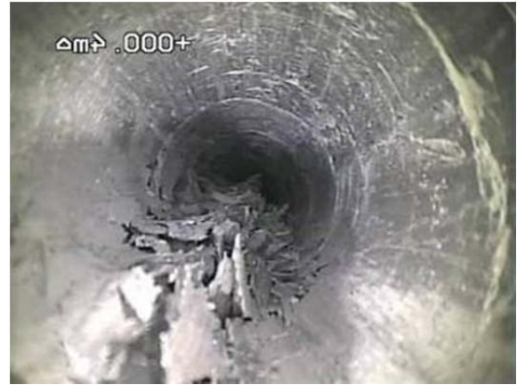
Fig. 11 Screenshots of borehole videos showing the progressive evolution of damage in a horizontal borehole following the bedding (Hesser et al., in prep.). Bedding planes dip \sim 45^\circ to the right. The images were flipped to allow comparison with Figure 10. Right image taken 3 months after left image at different depth positions. Left: shearing along bedding (black arrows) and incipient buckling in the background (white arrow). Right: fragment rotation in deeper regions pushes up the borehole contour to form a triangular structure; about a third to a half of the borehole circumference is affected by the failure
