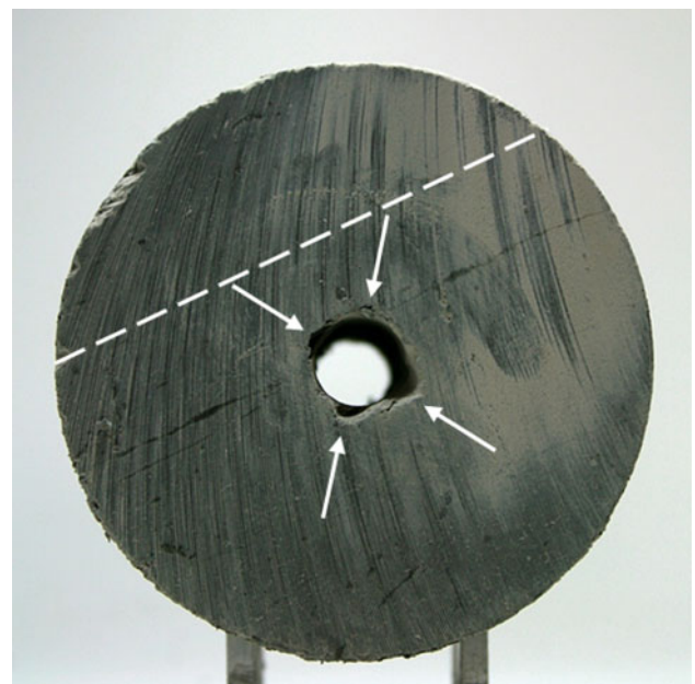
Fig. 5 Picture of the Opalinus Clay sample N°2/5 cored parallel to the bedding planes ( white dashed line ) after its removal from the testing cell and saw cutting. Early stage features of failure indicated by the arrows
