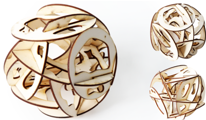
Figure 11: A lampshade design uses non-tight slits to facilitate a complex intersection pattern. Our optimization still guarantees that the assembled structure is completely rigid.
