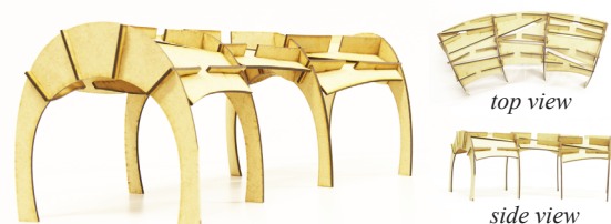
Figure 9: An architectural design study of an outdoor pavilion made from orthogonally intersecting pieces.
