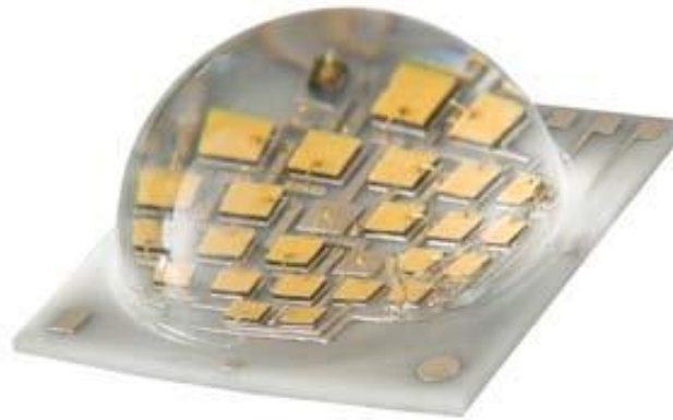
Figure 9.3: High power white LED CREE XLamp MP-L. The array of single emitters is visible under the polymer dome lens cover.
