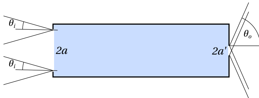
Figure 7.1: Schematic illustration of an angle transformer with acceptance half angle \theta_i , output angle \theta_o and the input and output aperture with diameter 2a and 2a' .
