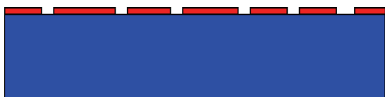
Figure 1. Fused silica substrate with a patterned poly-Si mask.
