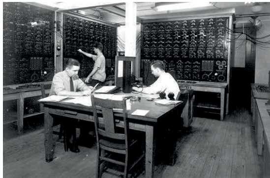
Figure 3.2.: 3 out of 5 blocks of the MIT network analyzer. Photo reproduced from [33]
