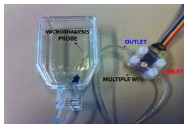
In-house chip holder in PMMA hosting the PDMS chamber and the biochip
