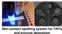
Non-contact spotting system for CNTs and enzyme deposition
