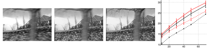
Fig. 1. Left to right: before registration; after registration with affine transformations; with smooth transformations; SNR vs. m/n for the proposed method with model 1 (dashed red), 2 (continuous black), 3 (continuous red), and the BP method (dashed black). The curves represent the mean SNR over 10 simulations, and the vertical lines the error at 1 standard deviation.
