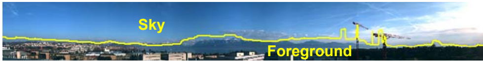
Figure 5.5: In this example, we consider the non-sky part as the region of interest (ROI). An automated algorithm can find the boundary (the yellow line) between the sky and the foreground buildings/mountains.
