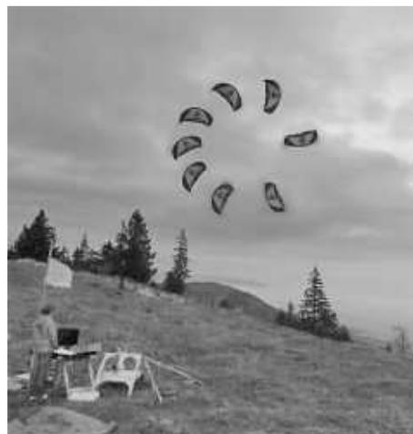
Fig. 1. A superimposed sequence of frames shows a kite following a closed path during testing of EPFL’s lab-scale system.
