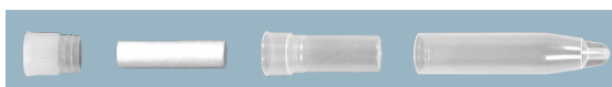
Figure 2.5: Swab saliva collection tool: Salivette ® system with stopper, swab, insert, and Salivette ® tube (left to right). [98]
