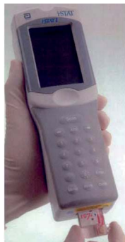
(a) iSTAT system for detection of electrolyte levels and limited immunoassays [22].
