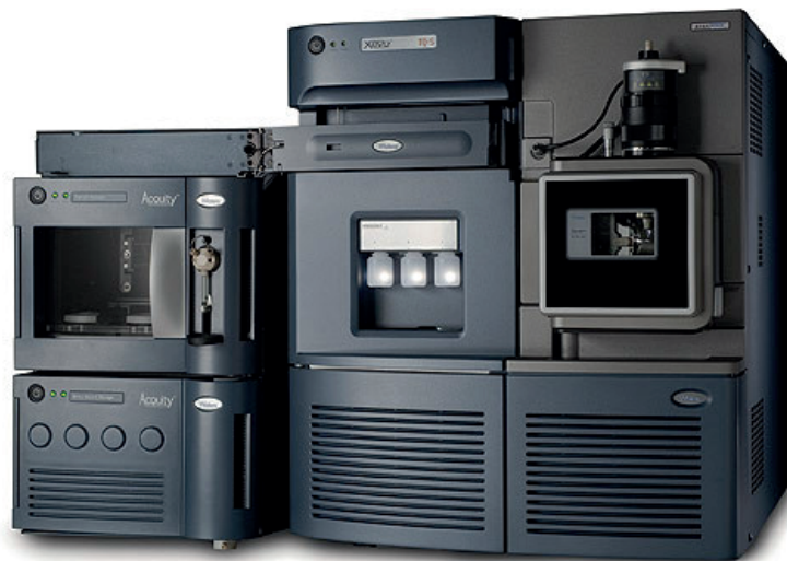
Figure 2.12: Ultra performance liquid chromatography - mass spectrometer Xevo TQ-S from Waters [113].
