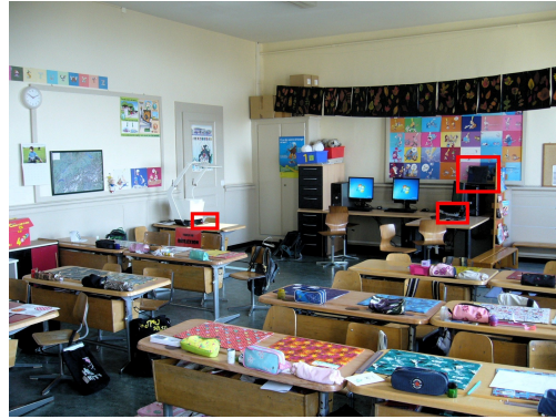
(b) Another laptop computer was placed on top of one of the classroom computers; its webcam filmed the class from the back. An ambient microphone was placed near the laptop in the back to capture the sound in the classroom. A panoramic camera was placed under the Metroscope.
