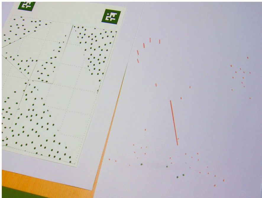
Figure 8.22: On the right: the range of feedback. From bottom to top: green dots (correct), red points (small imprecision), a long red line (detection artefact) and red lines (bigger imprecision).
