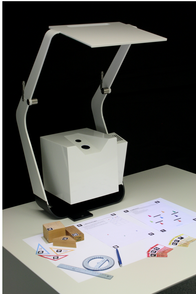
Figure 3.2: The Metroscope, our camera-projector system, along with various types of objects which can be augmented on a table: sheets, cards, tools and wooden blocks.
