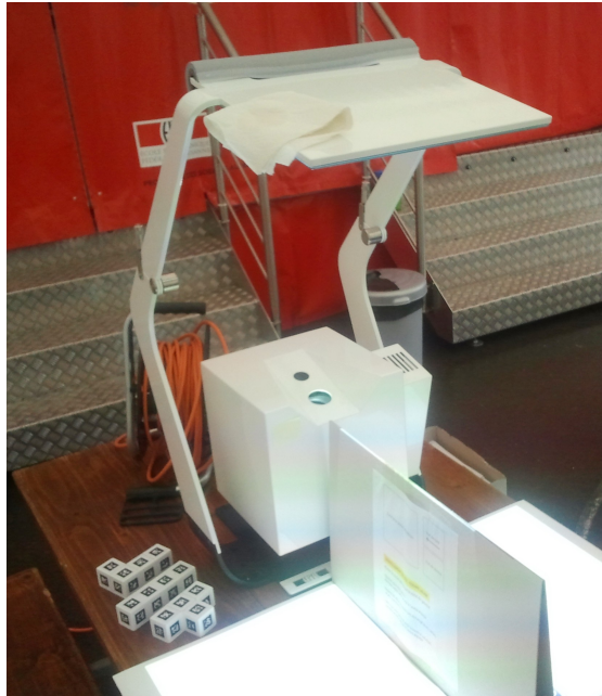
Figure 3.5: The Metroscope in less than ideal (lighting and humidity) conditions. Note the tissue on the top to absorb the water dripping from the roof of the tent.
