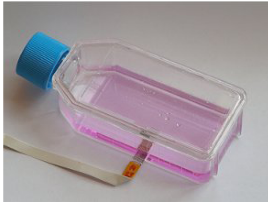
Figure 2.6: Cell culture flask with equipped with in situ sensor for the detection of nitric oxide. Reprinted from [16].
