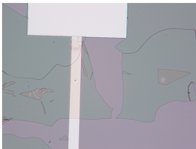
Figure 4.4: Magnified optical image of pads and connection after wet etching of SiO 2 .
