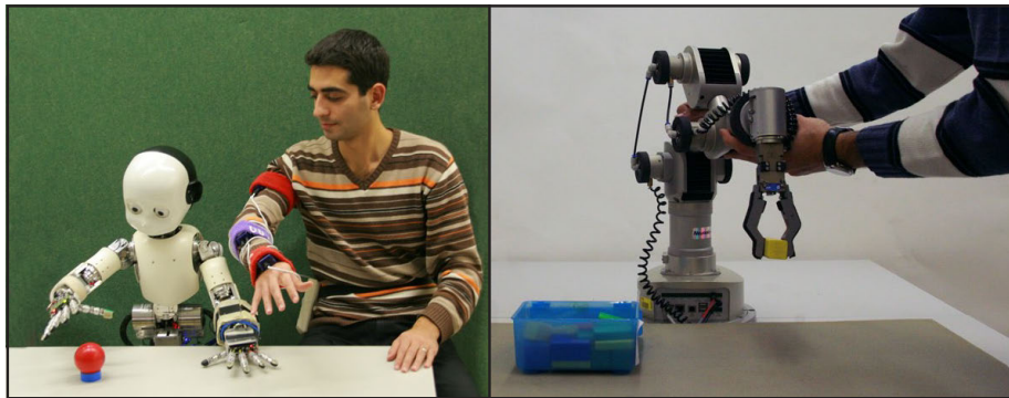
Figure 4.1: Demonstrating motions by teleoperating a robot using motion sensors ( left ) or by back-driving it ( right ).
