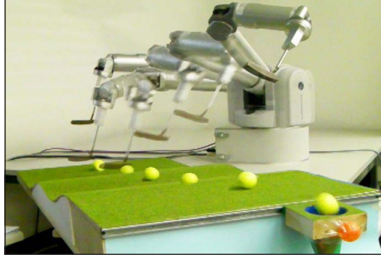
Figure D.6: The hitting motion on the WAM. The ball and the hole are continuously tracked by a stereovision system.
